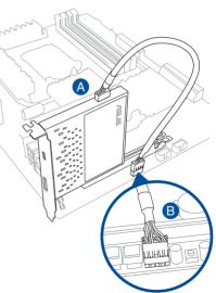
Connect the DisplayPort cable to the ThunderboltEX II card's DisplayPort IN port (A) and to the DisplayPort or mini DisplayPort on the motherboard's I/O port (B).
